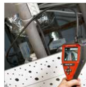
Camera head with high-performance LEDs
