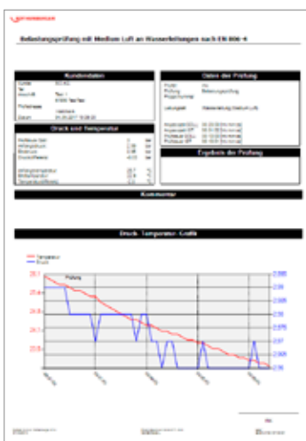
Sample log according to DIN EN 806-4 with measurement value table
