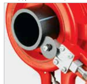
ROCUT 110 with cutter wheel (No. 54950) (special accessories)
