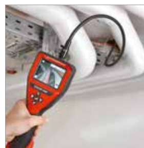
Inspection of hollow spaces
