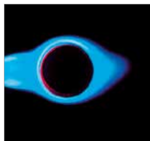
High flame temperature based on cyclone swirl
