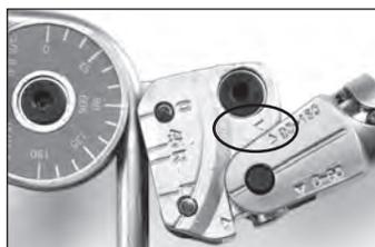
Figure 13 – Rotate Handle
